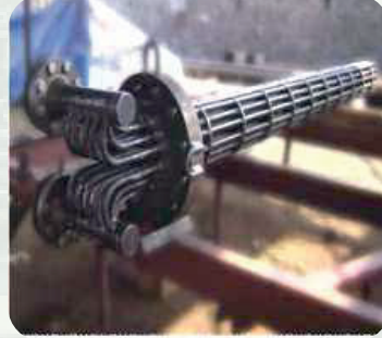
De-Super Heater Assembly
